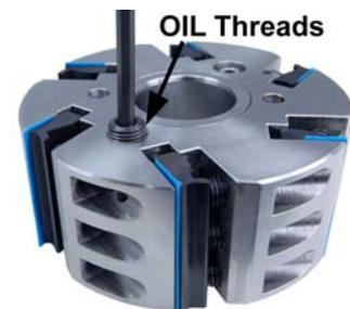
Easy lock heads are equipped with a set of filler grease nipples that can be used to re-pressurize the sleeve if required during an o-ring replacement. Note the filler nipple is not for use in everyday operation.
